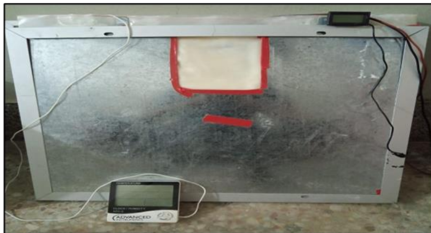
Figure II. Back side of the PV plate is equipped with an Aluminum sheet.
