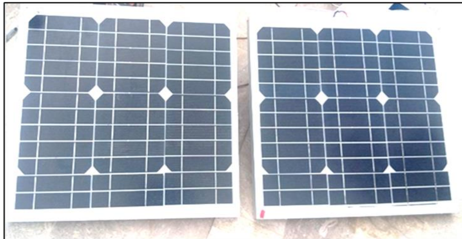
Figure I. Two panels, the right one is equipped with PCM while the left is without PCM.
