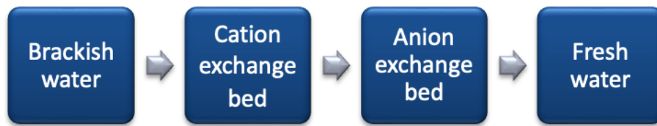
Figure III. Ion exchange process
