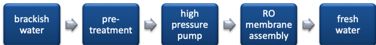
Figure II. Reverse Osmosis process.
