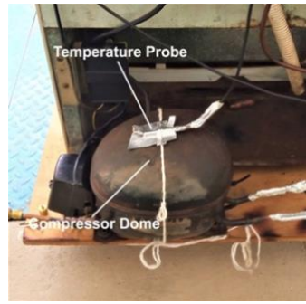
Figure IV. Placement of temperature sensors at compressor dome
