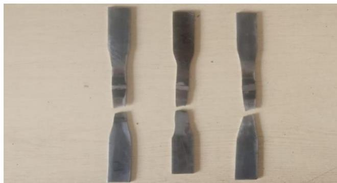
Figure IV: Tensile Testing Samples.
