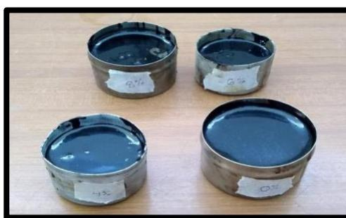
Figure I. Penetration Sample.
