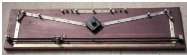
Figura V. Puente Wheatstone (Leeds and Northrup).
