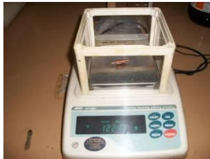
Figure IV. Precision weighing scale AND GF-200.
