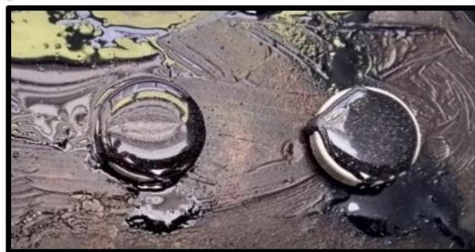
Figure III. Softening Point Sample.
