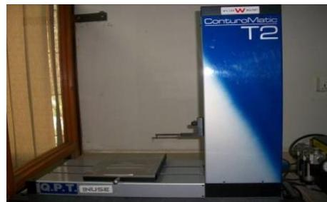
Figure V. Surface Roughness Tester WW CM T2.
