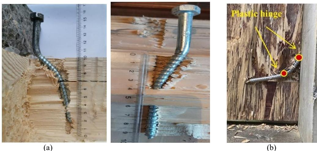
Figure VIII.- The failure mode of pushing out specimen and crushing deformation of timber
