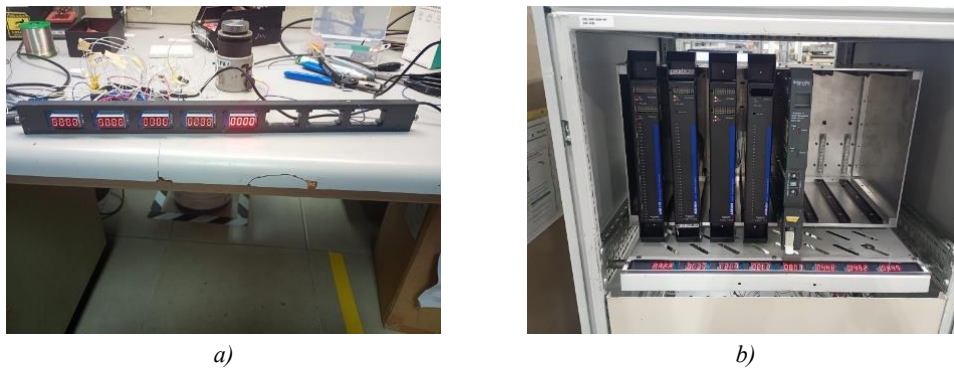
Figure V. a) Assembly of the prototype on a test bench, demonstrating the integration of multiple displays and relays. b) Installation of the prototype in the production line's test cabinet.
