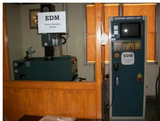
Figure 1. GENSARK EDM Machine used for EN-31 steel.
