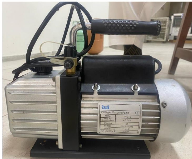
Figure VII.- Vacuum Pump for system evacuation
