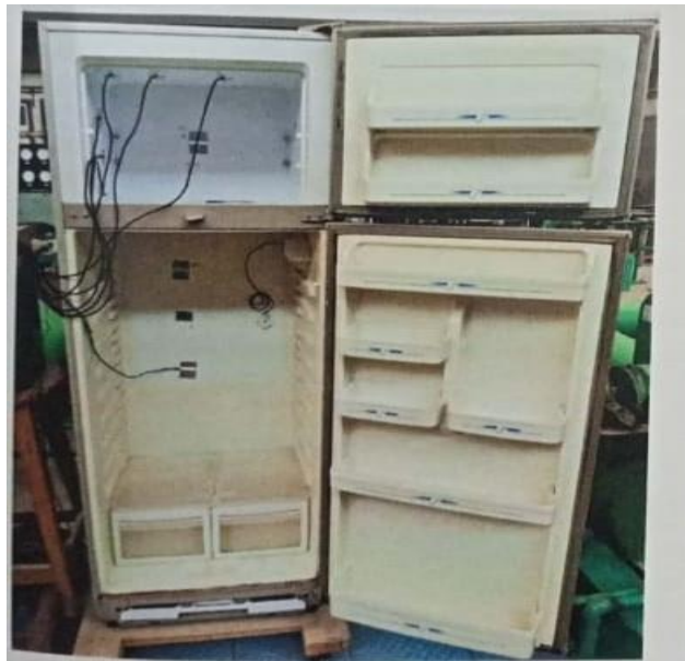
Figure III.- Refrigerator with Data logger Sensors
