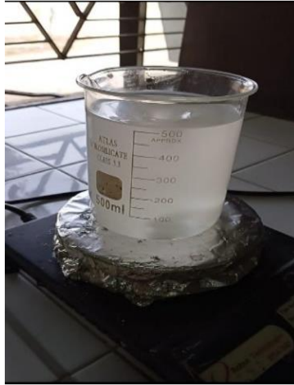
Figure I.- Beaker with magnetic stirrer placed on Hot plate
