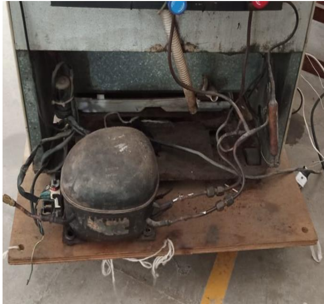
Figure IV.- Modified location of Compressor
