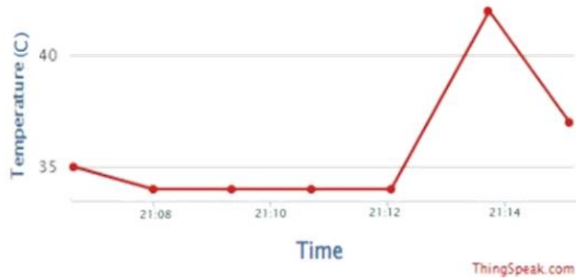
Figure VIII. Change in battery surface temperature due to change in current.
