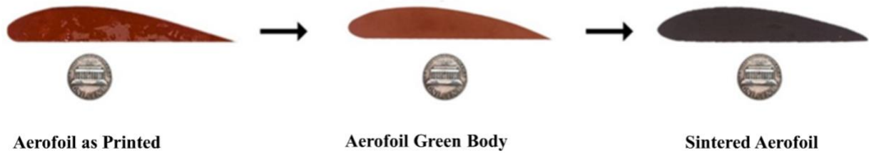
Figure III. Transformation from the DIW part to the sintered monolithic ceramic body (Aerofoil Geometry).
