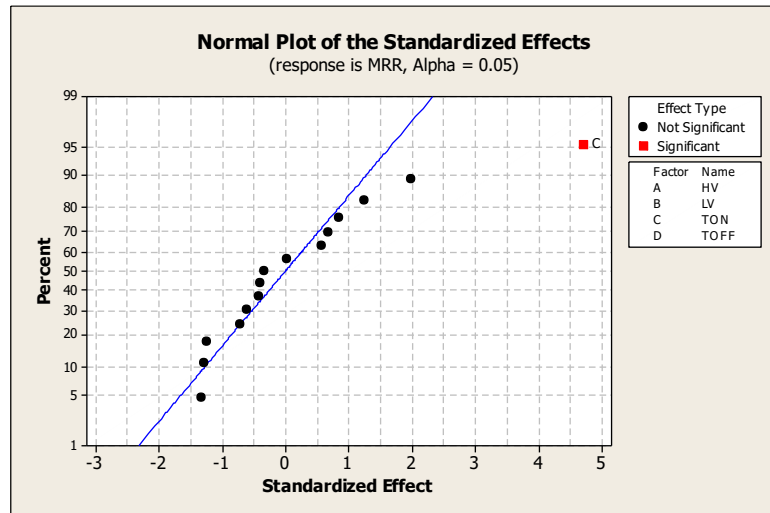
Figure IX. Normal Probability Plot of the standardized effects of MRR for EN-31 considering all factors
