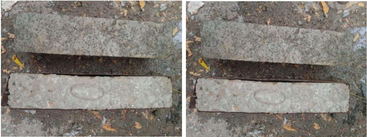
Figure III. Representation of concrete for flexural testing
