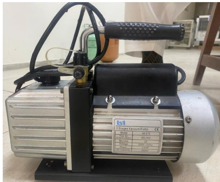
Figure VII.- Vacuum Pump for system evacuation
