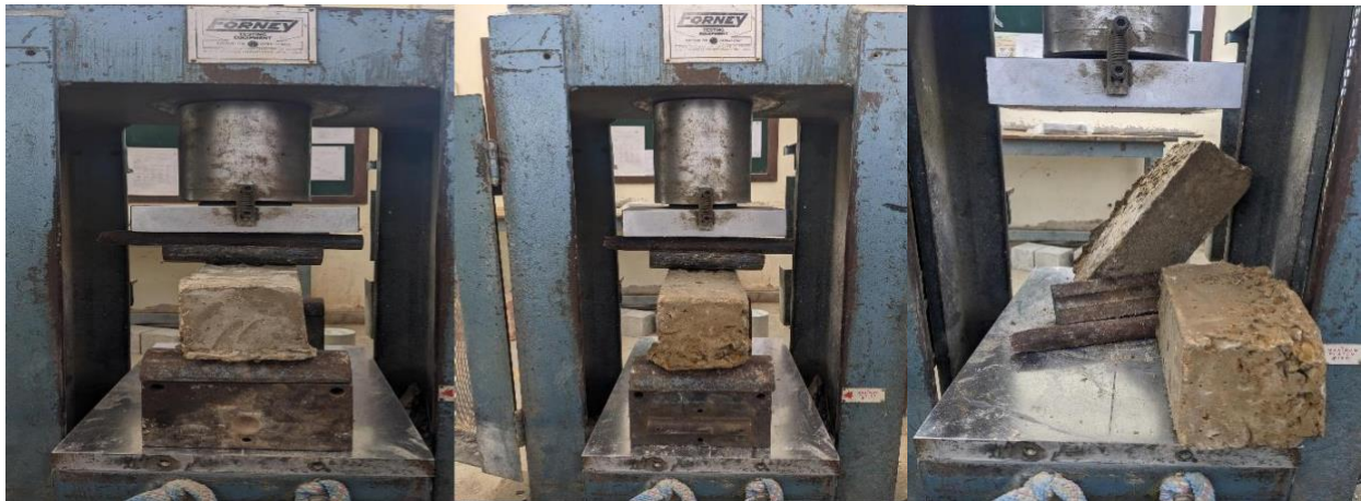
Figure VI. Experimental Setup of Flexural Strength Test of Concrete Specimens by UTM.
